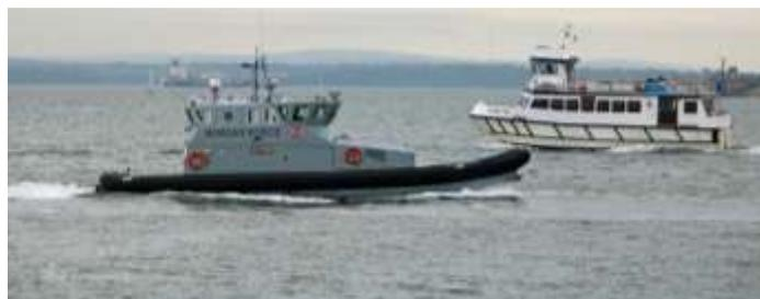
The Border Force has subsequently procured some Coastal Patrol Vessels as shown here – large RHIBs to you and I – with a 280 mile range at 20 knots and a top speed of 32 knots. A Freedom of Information reply gave the following information:
