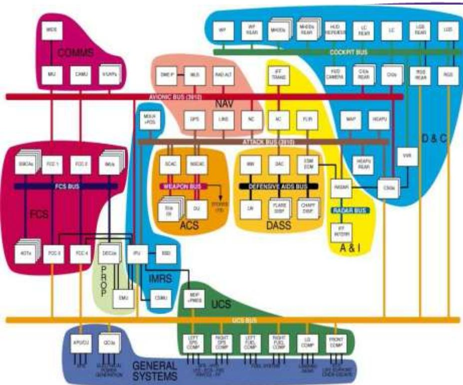
Typical Aircraft Avionic System Architecture
