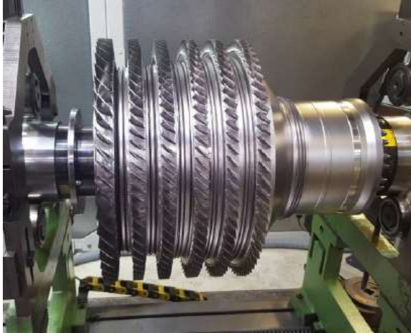
HPC without casing
